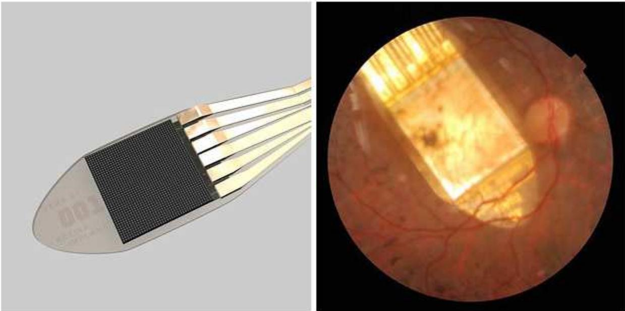
The small electronic chip implanted at the back of the retina to replace damaged photoreceptors. *University Of Oxford / Press Association Images*
